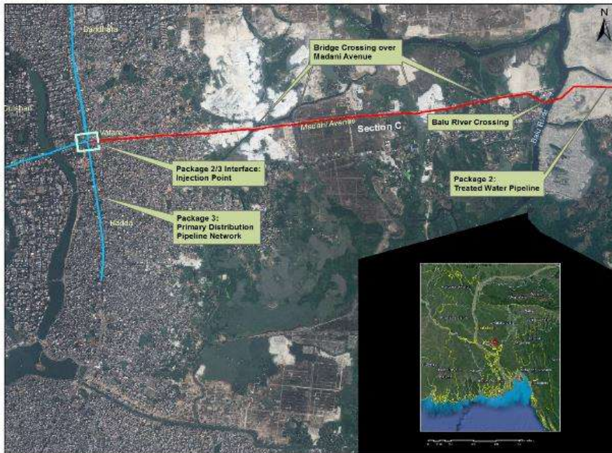
Figure 4-4: P2 Pipeline Route up to Injection Point
